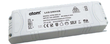
AT9644/60 SKU 11370 60W 24V DC Constant voltage Dimmable driver with Flex & Plug Dimensions: 170 x 50 x 29mm
