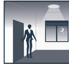
With insufficient ambient light, the sensor switches on the lamp when motion is detected
